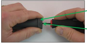
Align *Circuit Board Holding Tool* and insert fully into logger housing.
