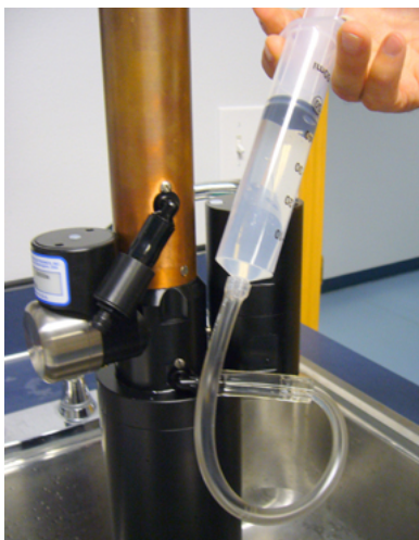
Figure 15 Triton® X-100 solution into the CT-DO
