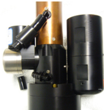
Figure 14 Exhaust tube removed from elbow fitting
