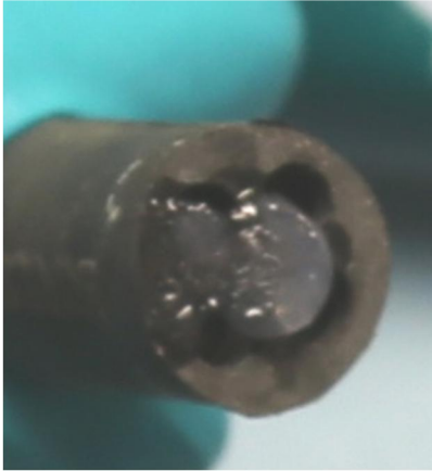
Lubricant on socket end of connector
