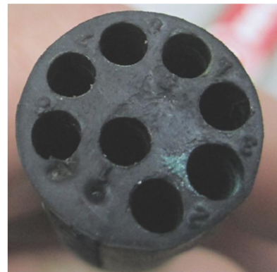
Damaged socket face
