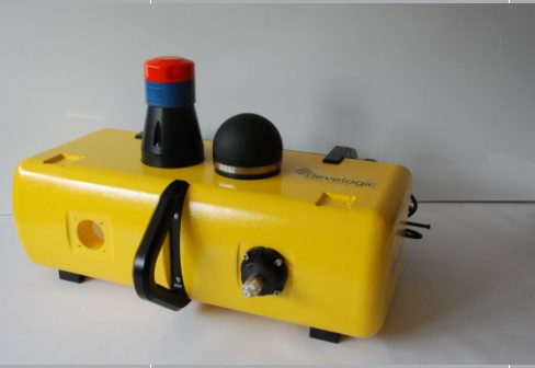
develogic modular seafloor lander with current sensor
